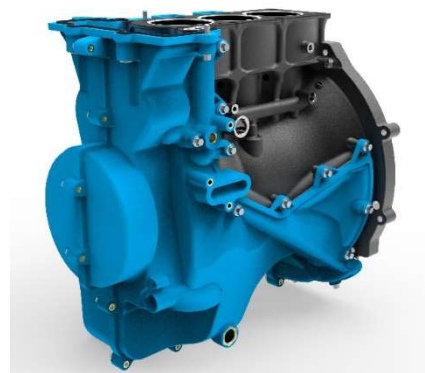
4(b) CGI cylinder block assembly with outer plastic casings
