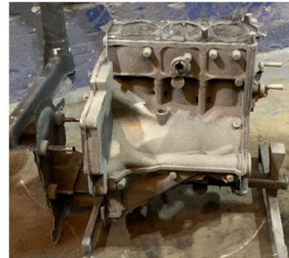
12(c) as-cast cylinder block with gating system and stabilizing bars
