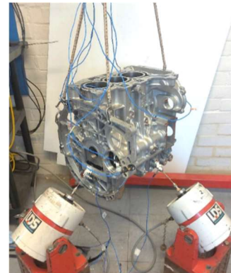
6(b) Aluminum block with upper and lower oil pans
