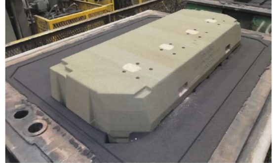
12(b) Assembled core package with four ladder-frames set into standard series production green sand flask
