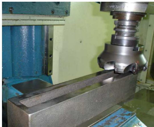
Fig. 2. The milling process used in the experimental work.
