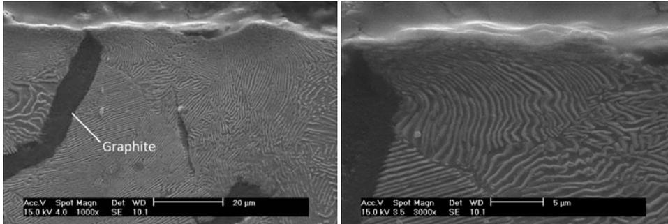
Notes:  $v_c = 1.400$  m/min. Modifications on the pearlitic matrix and on graphite and MnS particles.
