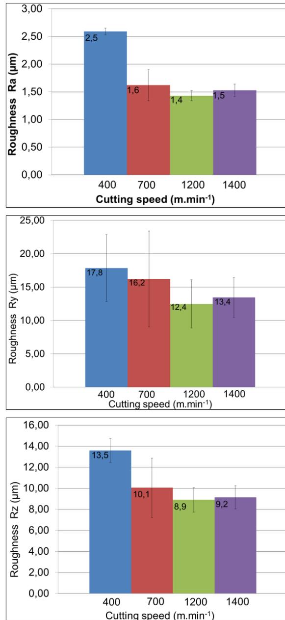
The results show that the roughness obtained at  $v_c = 400$  m/min is higher than those obtained at higher cutting speeds. This observation needs further confirmation, since the dispersions on the roughness value are very high. This behaviour agrees with previous studies in the literature (Boehs, 1979; Machado and Silva, 2004; Diniz et al., 2003). At the speed of 1,400 m/min it was found a small increase of roughness, which was
