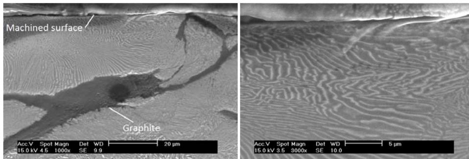
Notes:  $v_c = 400$  m/min. Modifications on the pearlitic matrix and extrusion of graphite particles.
