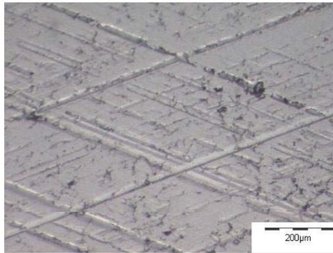
Note: Honed grooves and micro pores from the fracture of graphite.
