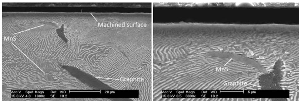
Notes:  $v_c = 1.200$  m/min. Modifications on the pearlitic matrix and on graphite and MnS particles.
