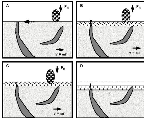
Notes: A – action of the normal force and graphite compression; B – surface runoff with graphite extrusion; C – volume collapse occupied by graphite; D – sealing by compressive residual stresses and wear.
