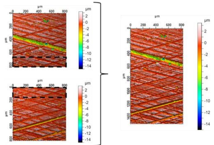
Figure 11. Stitching operation to join the surfaces.
