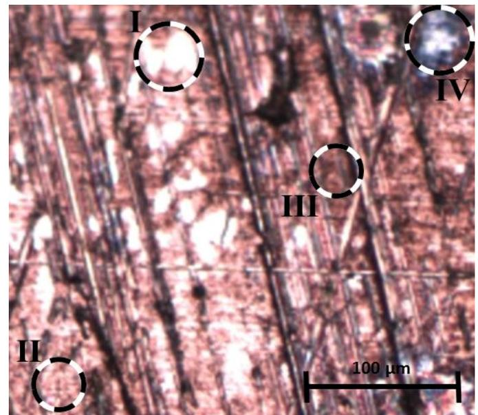
Figure 5. Positions at TDC in which oxides and tribofilms were analyzed (10x amplification).
