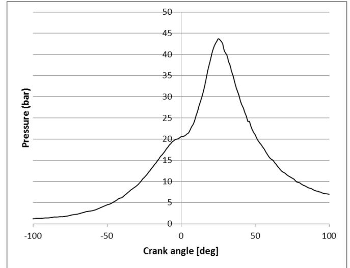
Figure 1. Pressure-crank angle diagram for compression and power strokes (1300 rpm).
