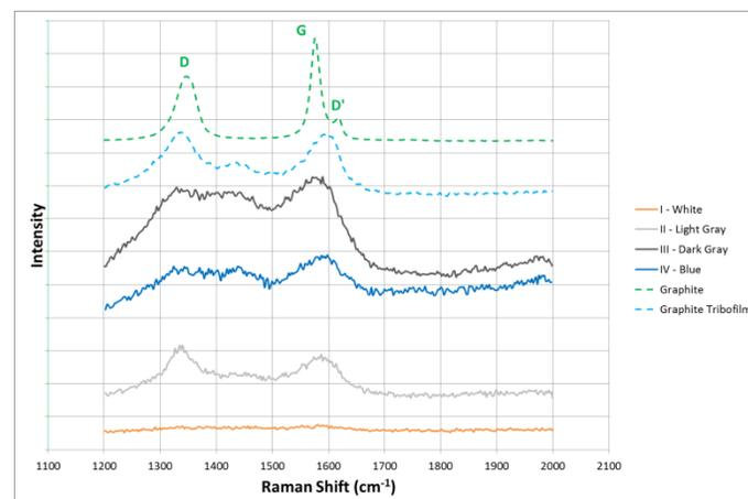
Figure 8. Raman spectra at TDC.
