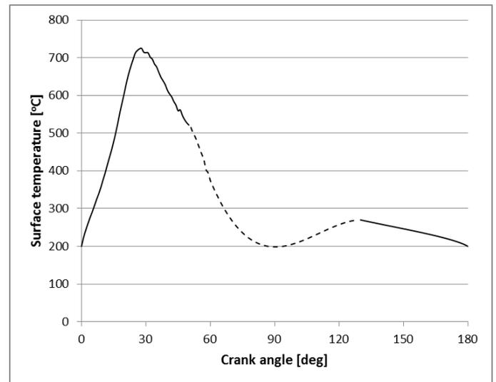
Figure 2. Temperature of the cylinder during power stroke.
