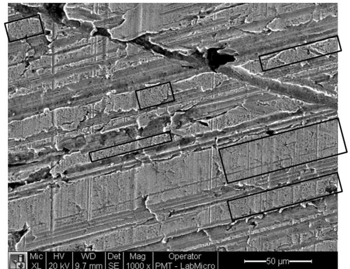
Figure 4. TDC of the honed surface showing corrosion pits.
