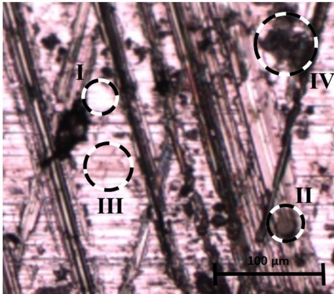
Figure 6. Positions in the mid-stroke region of the cylinder in which oxides and tribofilms were analyzed (10x amplification).
