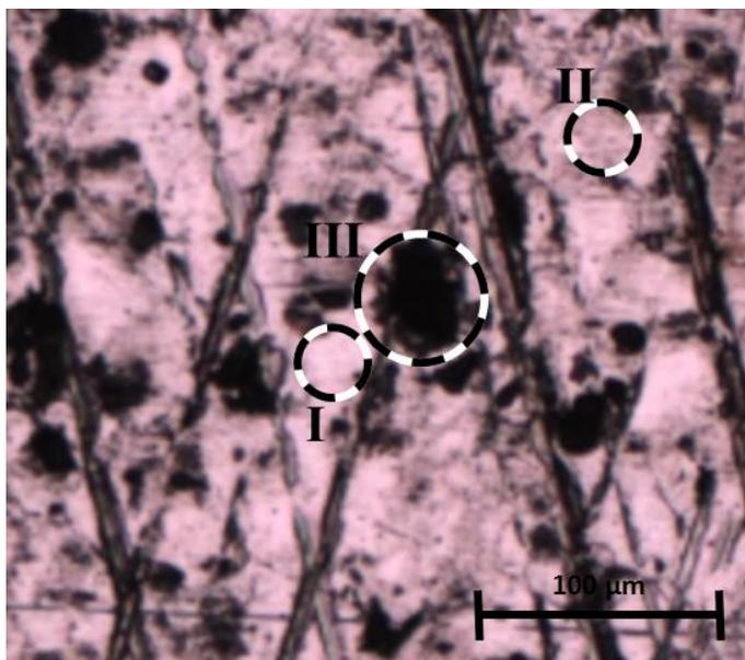
Figure 7. Positions at BDC in which oxides and tribofilms were analyzed (10x amplification).
